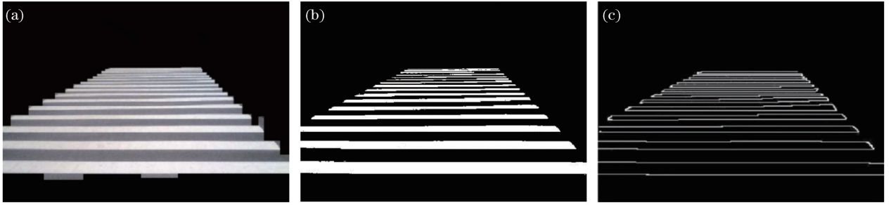
图6 斑马线特征提取结果。(a)原始图像中的目标区域;(b)阈值分割结果;(c)边缘提取结果 Fig. 6 Results of feature extraction for zebra crossing. (a) Candidate region in original image; (b) threshold segmentation result; (c) edge extraction result
