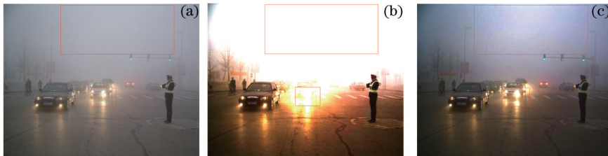
图2 图像增强结果对比。(a) 图像 traffic2; (b) 传统方法计算透射率; (c) 本文方法计算透射率 Fig.2 Contrast of image enhancement results. (a) Image traffic2; (b) transmittance with traditional method; (c) transmittance with proposed method
