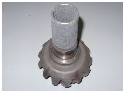
Fig.6 Laser direct manufacturing thin cylinder component
