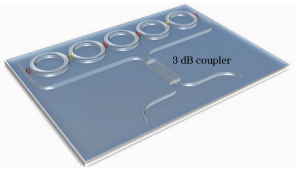
图 5 平面基板上微谐振环耦合结构集成光学陀螺 [43] Fig. 5 Illustration of micro-resonator CROW integrated optical gyroscope on planar substrate [43]
