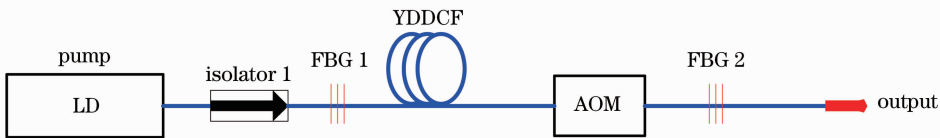
图 2 全光纤型声光调 Q 脉冲光纤激光器典型装置 Fig. 2 Typical setup of all-fiber AOM Q-switched pulsed fiber lasers
