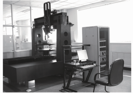
图 3 非球面数控加工中心 Fig. 3 Computer-controlled machine for manufacturing aspheric
