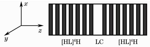
图 1 液晶缺陷一维光子晶体滤波器结构示意图 Fig. 1 Schematic diagram of one dimensional photonic crystal filter with liquid crystal layer
