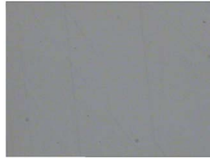
图6 抛光 20 min 后 K9 玻璃表面形貌( \times 1500 ) Fig.6 Morphology of K9 glass after 20 min polishing ( \times 1500 )
