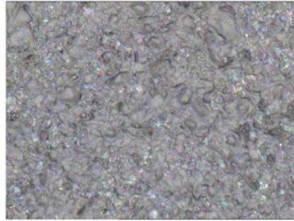
图 3 抛光前 K9 玻璃表面形貌( \times 1500 ) Fig.3 Morphology of K9 glass before polishing ( \times 1500 )
