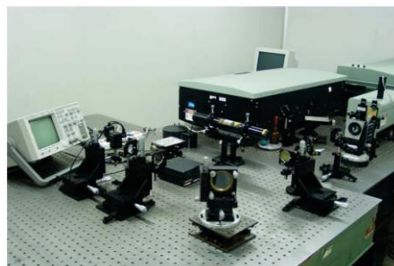
图 4 脉冲光腔衰荡高反射率测量实验装置照片 Fig.4 Experimental setup of pulsed-CRD for high reflectivity measurements
