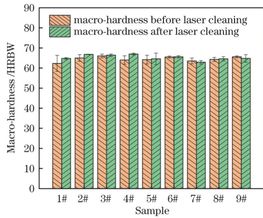
图 10 未清洗试样与在参数 1 # ~9 # 激光清洗后试样的宏观硬度 Fig.10 Macro-hardnesses of uncleaned sample and samples after laser cleaning under parameters 1 # -9 #
