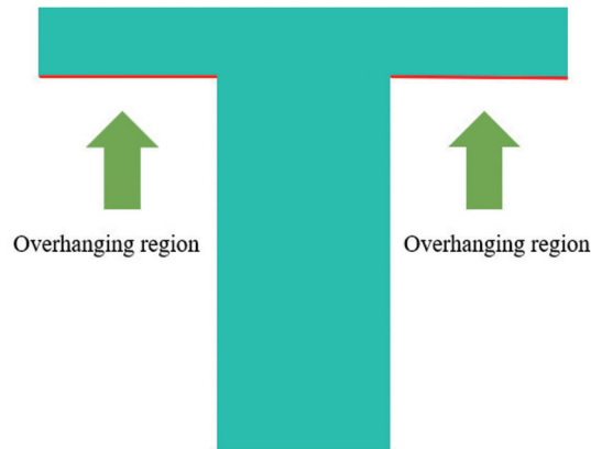
图1 悬垂结构示意图,其中红色区域为悬垂结构区域 Fig. 1 Schematic diagram of the overhanging structure, where the red areas is the overhanging structure areas
