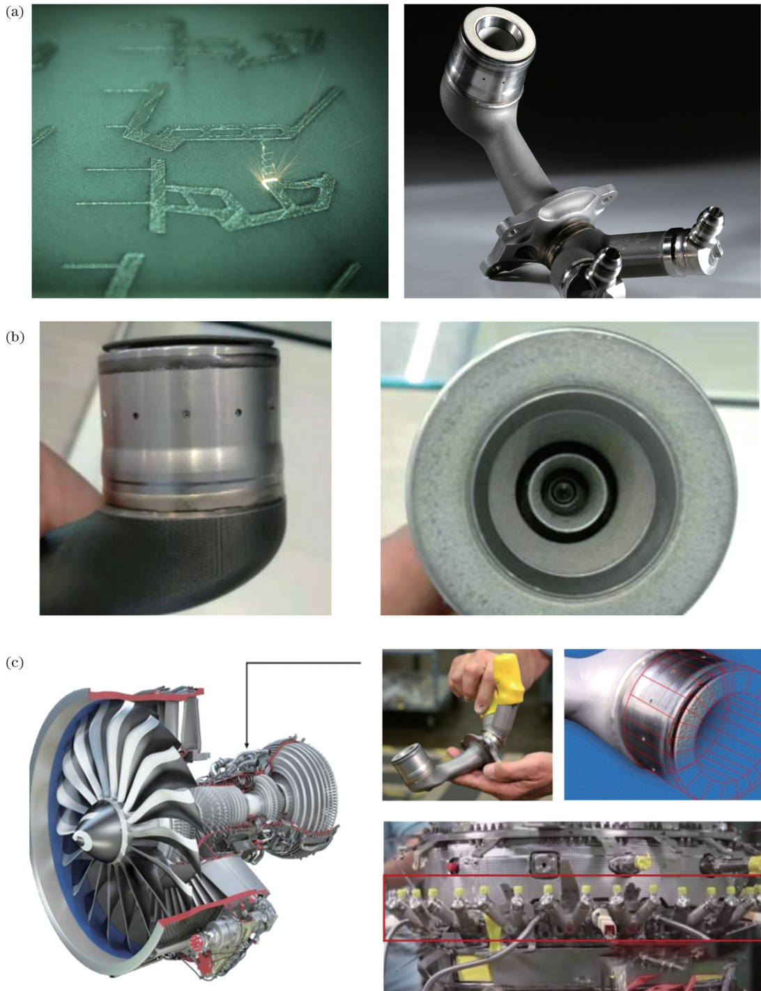
图 10 GE 公司利用增材制造技术制造燃油喷嘴 [48] 。(a)燃油喷嘴 LPBF 成形;(b)喷嘴端部迷宫式复杂流道;(c)燃油喷嘴性能测试 Fig. 10 Development of fuel nozzles by GE using AM [48] . (a) LPBF forming of fuel nozzles; (b) labyrinth-type complex flow channel on nozzle end; (c) performance test of fuel nozzles
