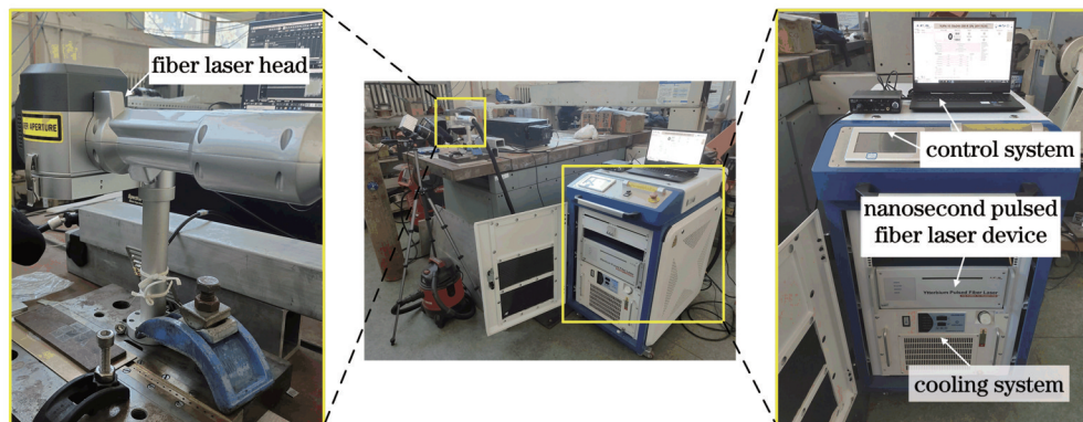
图 2 激光清洗系统实景图 Fig. 2 Photographs of laser cleaning system
