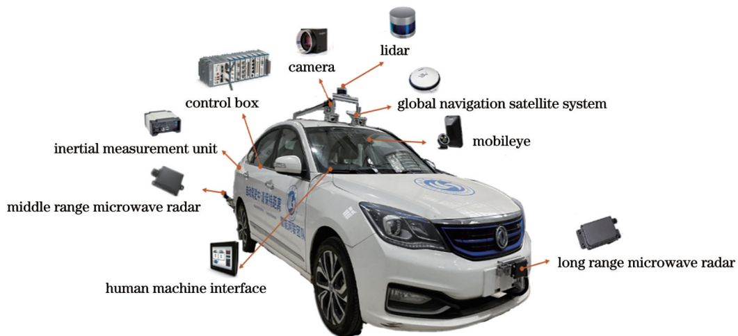
图 7 实验平台车的硬件部署 Fig. 7 Hardware deployment of experimental platform vehicle
