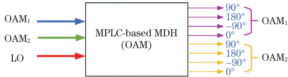
图 14 OAM 模的模解复用混频输入-输出端口示意图 Fig. 14 Schematic of mode demultiplexing mixing input-output port of OAM mode
