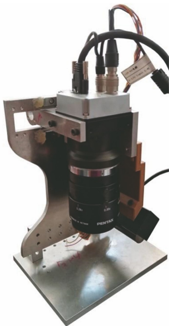
图 4 激光清洗表面在线检测设备 Fig. 4 Online detection mechanism of laser cleaning surface
