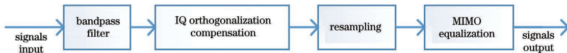
图 4 基于 LMS-MIMO 算法的离线处理步骤 Fig. 4 Offline processing steps based on LMS-MIMO algorithm
