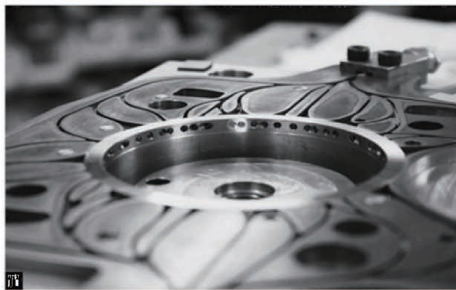
图 12 非规则 27 路的固定光路传感器 Fig. 12 Sensor with 27 fixed optical paths irregularly designed
