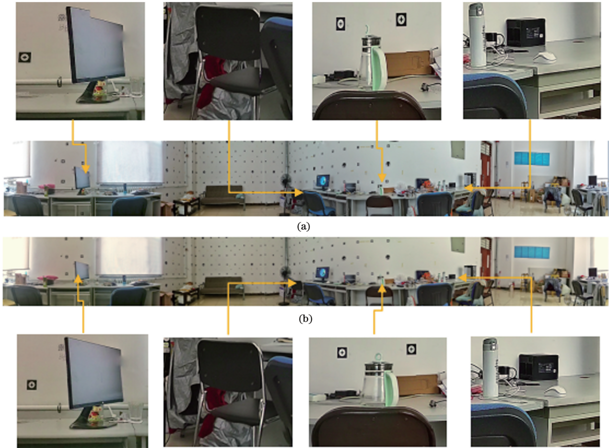
图 5 一个圆柱和多个圆柱全景拼接方法。(a) r=3989.4 mm; (b) r_1=1510 mm, r_2=2300 mm, r_3=2900 mm, r_4=2300 mm, r_5=1480 mm, r_6=2100 mm, r_7=2930 mm, r_8=2780 mm Fig. 5 Single-cylinder and multiple cylinders panoramic stitching methods. (a) r=3989.4 mm; (b) r_1=1510 mm, r_2=2300 mm, r_3=2900 mm, r_4=2300 mm, r_5=1480 mm, r_6=2100 mm, r_7=2930 mm, r_8=2780 mm
