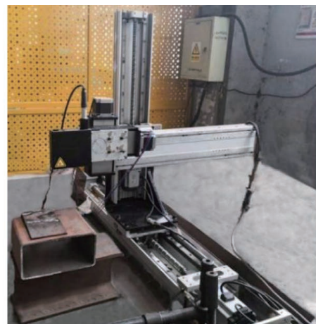
图 1 基于线结构光的焊缝表面质量检测实验装置图 Fig. 1 Experimental device of weld surface quality detection based on line structured light
