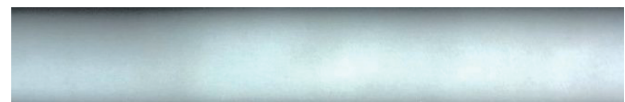
图 9 20 mm 厚 TC4 钛合金接头 X 射线底片 Fig. 9 X-ray film of 20 mm TC4 titanium alloy joint
