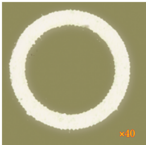
图 9 优化工艺条件下刻蚀图形阵列单元的显微照片 Fig. 9 Micrograph of etched pattern array elements under optimized process conditions
