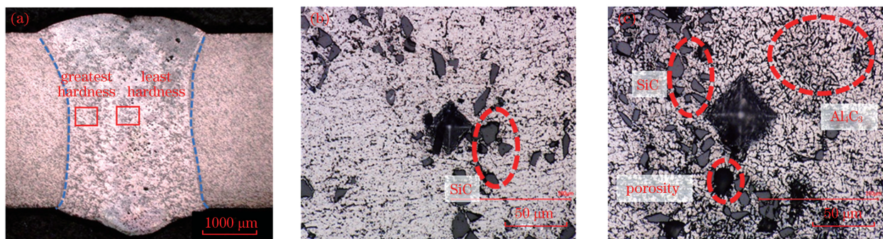
图 8 单光束激光填丝焊接接头的显微硬度分布。(a)焊缝截面;(b)硬度最大的位置;(c)硬度最小的位置 Fig. 8 Microhardness distribution of single laser beam welding with filler wire welded joints. (a) Weld section; (b) position of the greatest hardness; (c) position of the least hardness
