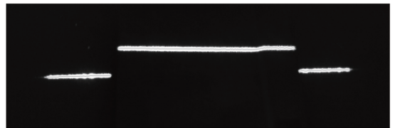
图 9 本文算法提取的光条中心 Fig. 9 Stripe centers extracted by the proposed algorithm
