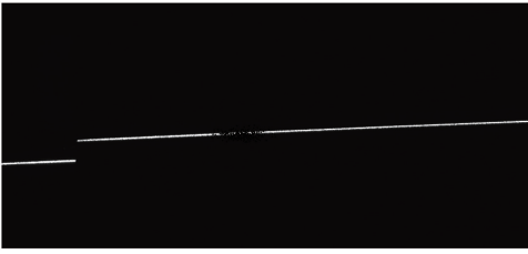
图 1 受被测物体表面污损影响发生断裂的激光条纹(模拟) Fig. 1 Laser stripe that breaks due to surface contamination of the object being measured (simulation)
