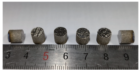
图1 激光选区熔化成形CP-Ti和Ti-5%TiN样品的宏观图片 Fig. 1 Macro picture of SLM-produced CP-Ti and Ti-5%TiN
