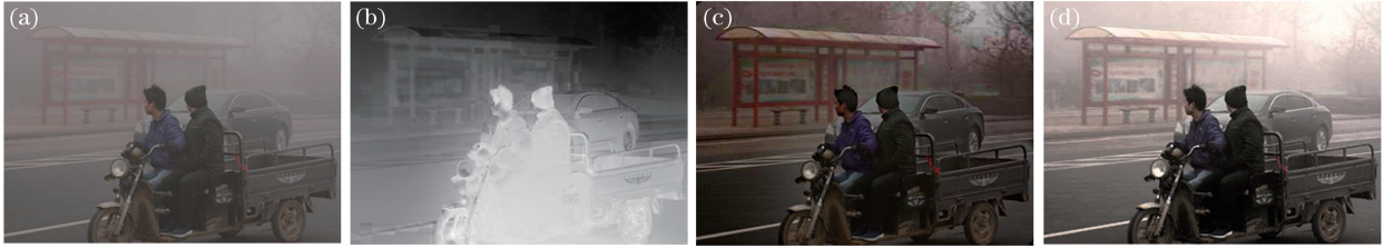
图 1 去雾图像实例。(a)输入图像;(b)归一化透射率图;(c)中值滤波的暗通道先验去雾图;(d) HSI 空间双直方图均衡图像 Fig. 1 Example of dehazed images. (a) Input image; (b) normalized transmittance image; (c) dehazed image based on dark channel prior with median filtering; (d) enhanced image using bi-histogram equalization in HSI
