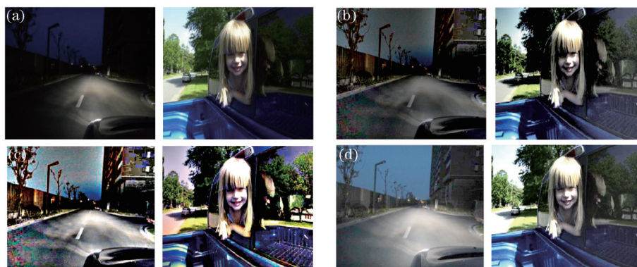
图5 三种算法在光照不均条件下处理结果比较。(a) 原始图像; (b) SSR算法; (c) MSR算法; (d) 本文算法 Fig.5 Comparison of processing results of the three algorithms under non-uniform illumination condition. (a) Original images; (b) SSR algorithm; (c) MSR algorithm; (d) the proposed algorithm
