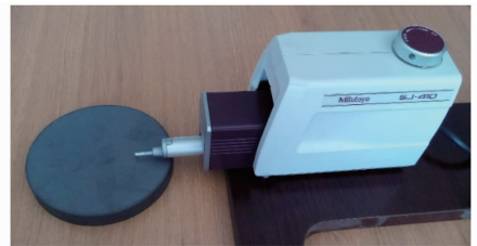
图 10 Mitutoyo SJ-410 测试 100 mm 口径 SiC 样片粗糙度 Fig. 10 Testing SiC sample surface roughness of 100 mm aperture with Mitutoyo SJ-410
