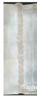
图 6 60 mm 厚 304 不锈钢窄间隙激光焊接接头横截面 Fig. 6 Section view of the welds of 60 mm thick 304 stainless steel achieved by narrow gap laser beam welding
