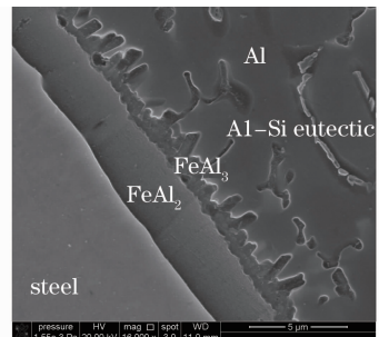
图 4 钢一侧连接界面处的 SEM 图像 Fig. 4 SEM image of joining interface at a side of steel
