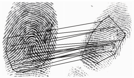
图 11 存在严重变形的一对指纹光学匹配结果 Fig. 11 Optically matched minutiae pairs between two fingerprints with large deformation
