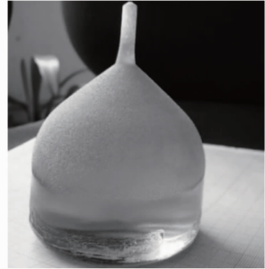
图1 温梯法生长出的Nd,Y:CaF 2 晶体照片 Fig. 1 Photo of as-grown Nd,Y:CaF 2 crystal obtained by TGT method
