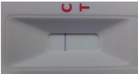
图 7 低浓度金标试纸条的实物图(0.5 ng/mL) Fig. 7 Photo of colloidal gold LF strip with low concentration (0.5 ng/mL)
