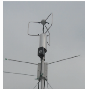
图 4 81000 型杨氏超声风速仪与 QHTP-2 型温度脉动仪实验图 Fig. 4 Experimental figure of Young's model 81000 ultrasonic anemometer and QHTP-2 temperature fluctuation instrument
