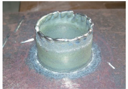
图 4 缺少高度控制导致表层凹凸起伏的堆积件 Fig. 4 Accumulation of surface fluctuations without height control
