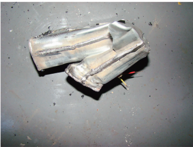
图 12 某车身三维零部件电弧焊碰撞试验结果 Fig. 12 Crash test result of an arc welding three-dimensional body part
