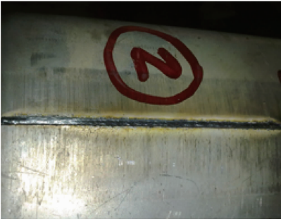
图 9 某车身三维零部件激光对接焊焊缝 Fig. 9 Laser butt joint weld of a three-dimensional body part
