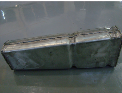
图 11 某车身三维零部件电弧对接焊焊缝 Fig. 11 Arc butt joint weld of a three-dimensional body part
