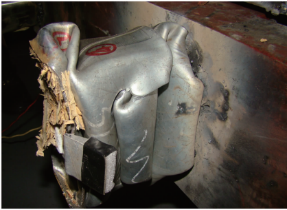
图 10 某车身三维零部件激光焊碰撞试验结果 Fig. 10 Crash test result of a laser welding three-dimensional body part
