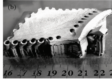
图 7 采用变密度成型工艺(a)以及采用致密态成型工艺(b)分别成型的两个手术导板 Fig. 7 Two surgical guide plates manufactured by (a) variable density rapid manufacturing process and (b) near-full-density producing process
