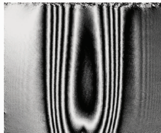
(e) cosine of unwrapped phase by shearing
