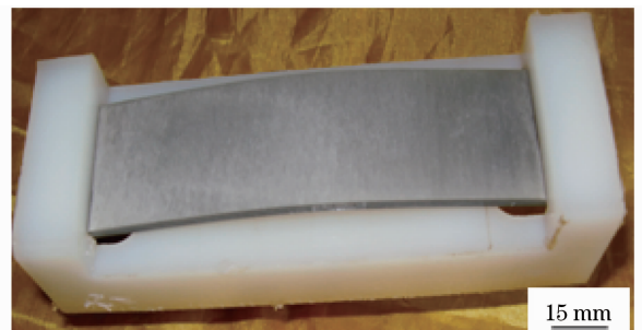
图 5 激光冲击试样应力腐蚀的结果 Fig. 5 SCC results of sample with LSP
