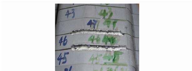
图8 入射角超过 $20^\circ$ 时的切缝Fig. 8 Kerf obtained when incident angle surpass  $20^\circ$
