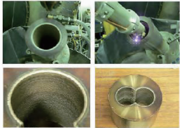
Fig. 8 Photographs of test sections for a 60-mm diameter single bore barrel (above) and a 60-mm twin bore barrel (below)
