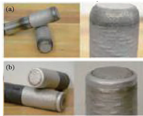
Fig. 5 Extrusion punch tools LAM clad with (a) NT-60 and (b) CCW-plus
