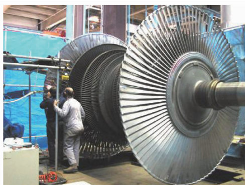
Fig. 1 Typical low pressure stage from a 200-MW turbine showing the blades
