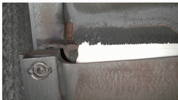
Fig. 2 Erosion of the blade after some eight to ten years of operation
