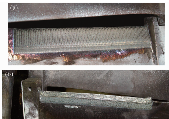
Fig. 4 Laser clad blades with (a) front view and (b) rear view before processing to original profile
