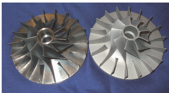
Fig. 22 Demonstration impellers with LC IN-718 blades built on pre-machined substrates. Left one in as-consolidated condition, and right one after sand blasting
