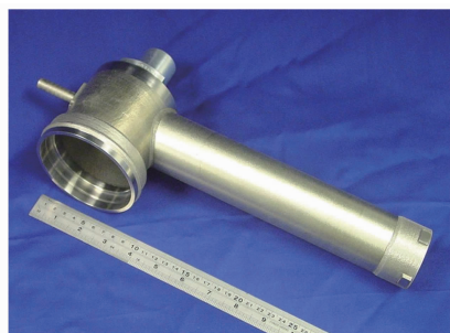
Fig. 18 LC Ti-6Al-4V integrated boom/housing, after initial machining
