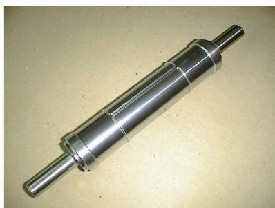
Fig. 14 LC CPM-9V rotary cutting die after final sharpening
