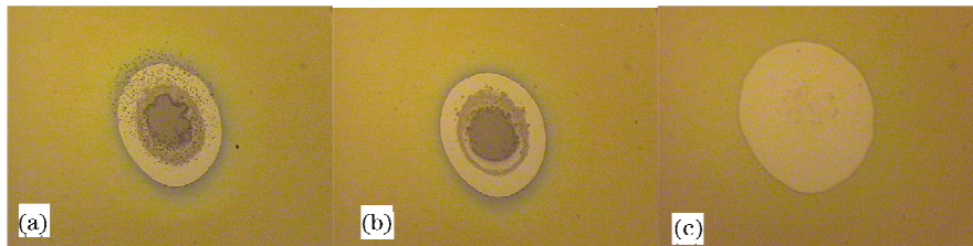
图 9 在相同的激光能量下真空和氮气环境下增透膜的损伤形貌。(a)真空;(b) 2 \times 10^{-2} Pa 的氮气;(c)1 Pa 的氮气 Fig. 9 Damage morphologies of ARF irradiated by the same laser energy under vacuum and nitrogen. (a) Vacuum; (b) 3 \times 10^{-2} Pa N_2 ; (c) 1Pa N_2
