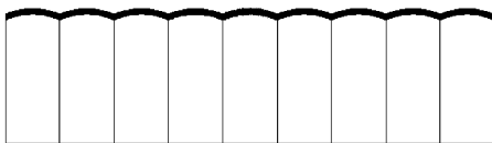
图 1 纵向侧面上刻有一列弧形槽的 D 型光纤 Fig. 1 D-type fiber with a series of longitudinal arc grooves on its side
