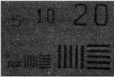
图 4 分辨率图像(绿激光直径 5 mm, 扫描步长 5 \mu\text{m} ) Fig.4 Resolution image obtained when green laser diameter is 5 mm and the scanning step is 5 \mu\text{m}
