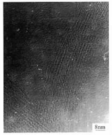
图 2 单壁碳纳米管束的高分辨透射电镜图 Fig. 2 HRTEM image of SWNTs produced by CO 2 continuous laser ablation
