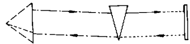
图 5 定向棱镜腔在激光棒热变形后的振荡光路 Fig. 5 Oscillating trace in directional prism cavity after crystal top deformed
