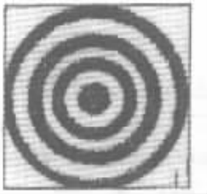
图1 均布载荷圆盘的离面变形条纹 Fig.1 Simulated fringe pattern
